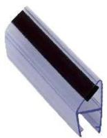
Made of Co-Extruded Plastic With Soft Magnetic Receiver. Provide Positive Door Closure, Mix and Match Configurations to Achieve Desired Result. Standard length 2200mm. Suitable to use on 10 & 12mm thick glass.
