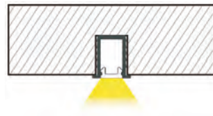
2. Recessed mounted, or install with glue
